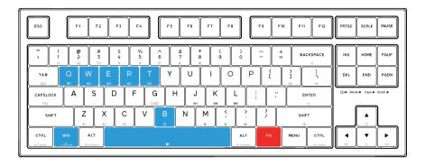
FN+Q: Profile 1 FN+W: Profile 2 FN+E: Profile 3 FN+R: Profile 4 FN+T: Profile 0
