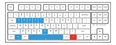
FN+B: Press long until light of the keyboard blinks, the keyboard reset to the factory default settings.
