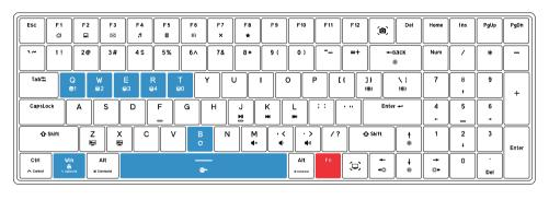
Fn+Q: Profile 1 Fn+W: Profile 2 Fn+E: Profile 3 Fn+R: Profile 4 Fn+T: Profile 0
